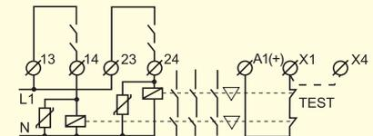
Contactors, relays and valves can be supervised by connecting 'test' contacts between A1(+) and X1. Both manual supervised and automatic reset can be used.
