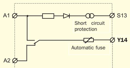
The RT9 should be supplied with +24 V on A1 and 0 V on A2.
